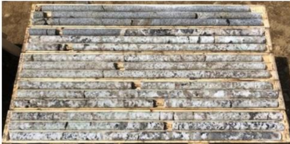
Figure 2 Spodumene pegmatite, 1.31 – 23.18 m, drill hole PWM-22-135, Main Dyke, Case Lake Property.
