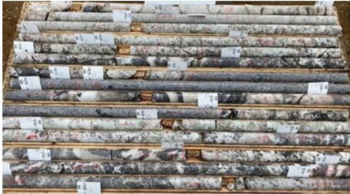
Figure 1 Spodumene pegmatite, 26.9-53.0 m, drill hole PWM-22-134, Main Dyke, Case Lake Property.
