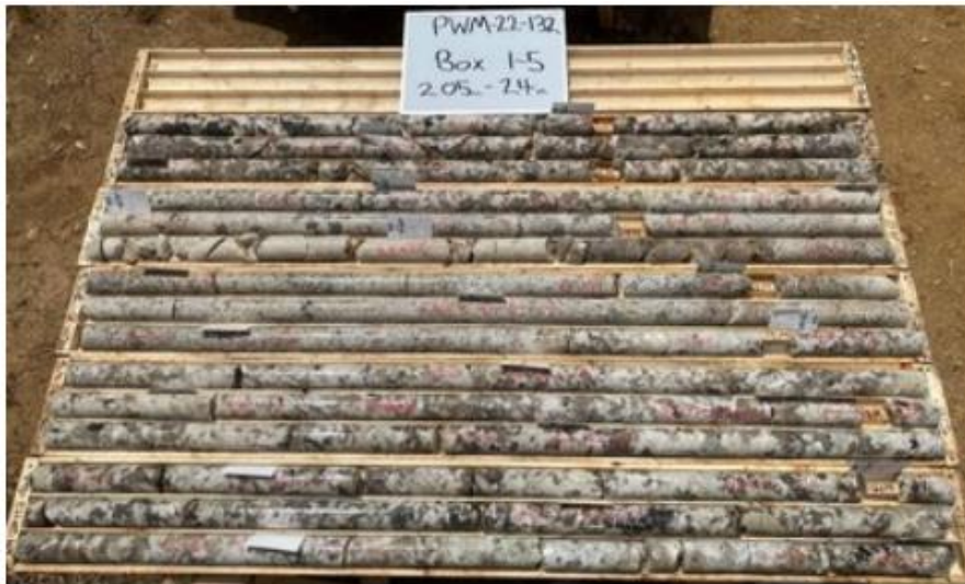
Figure 2 - Spodumene pegmatite, Main Dyke, drill hole PWM-22-132.
