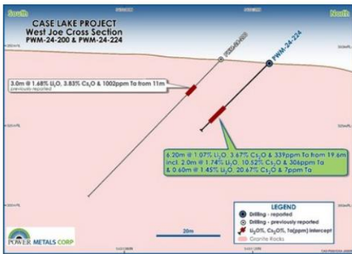
Figure 3 – Cross Section Map of PWM-24-224 from Phase II Drilling at West Joe (CNW Group/Power Metals Corp.)
