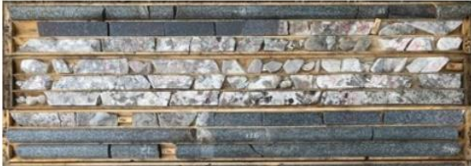
Figure 1 - Pollucite-spodumene-Ta-oxides West Joe Dyke pegmatite, Case Lake
