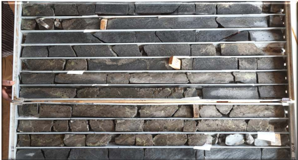
Figure 9: High grade Ni-Cu massive sulfide mineralization (SM44-454265 (2021-010) showing sharp contacts with the mineralized pyroxenite host.
