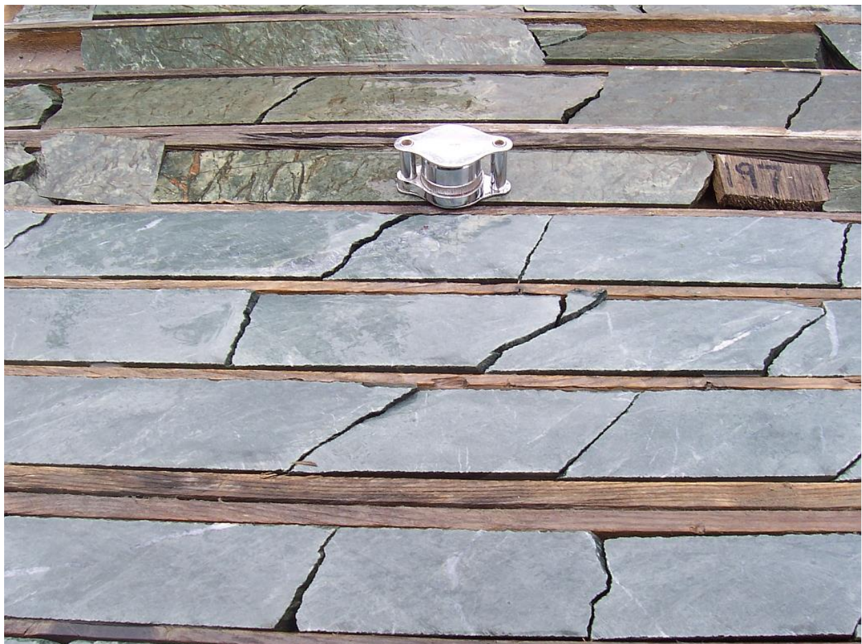
Photo of drill core from hole GB-05-2 showing weathered original sampling at top and recently cut core with quartz-carbonate veinlets, sericite alteration and disseminated pyrite.
