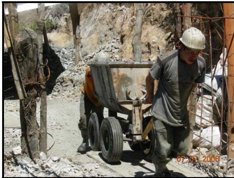
Photo 8: Hand pushed carts moving mineralized muck
