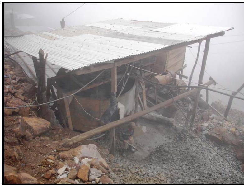
Photo 10: Los Incas trapiche (Chilean) milling equipment
