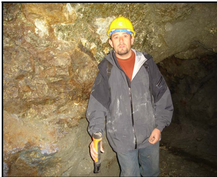
Photo 4: Diatreme breccia completely replaced by massive polymetallic sulphides, 3C-B stope, Los Humildes tunnel
