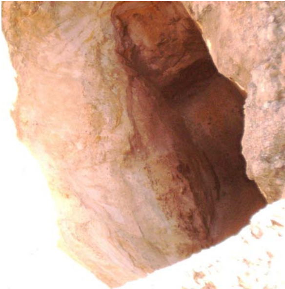
Photo 16 TH335 0.1-2.5' Gravelly clay 2.5-3.0' Gravel 3.0-20' Sand
