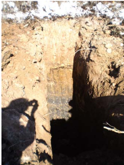
Photo 19 TH337 0.1-3.5' Gravelly clay 3.5-3.6' Dark layer of gravel 3.6-12' Oilsands
