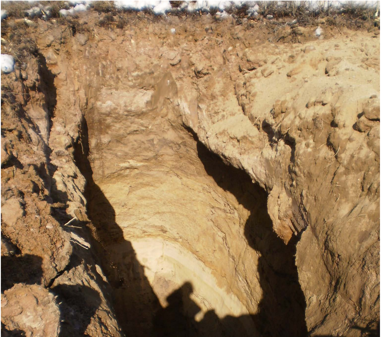
Photo 9 Test Pit TH322 0.1-8.2' Coarse dark sand 8.2-20' Light coloured sand
