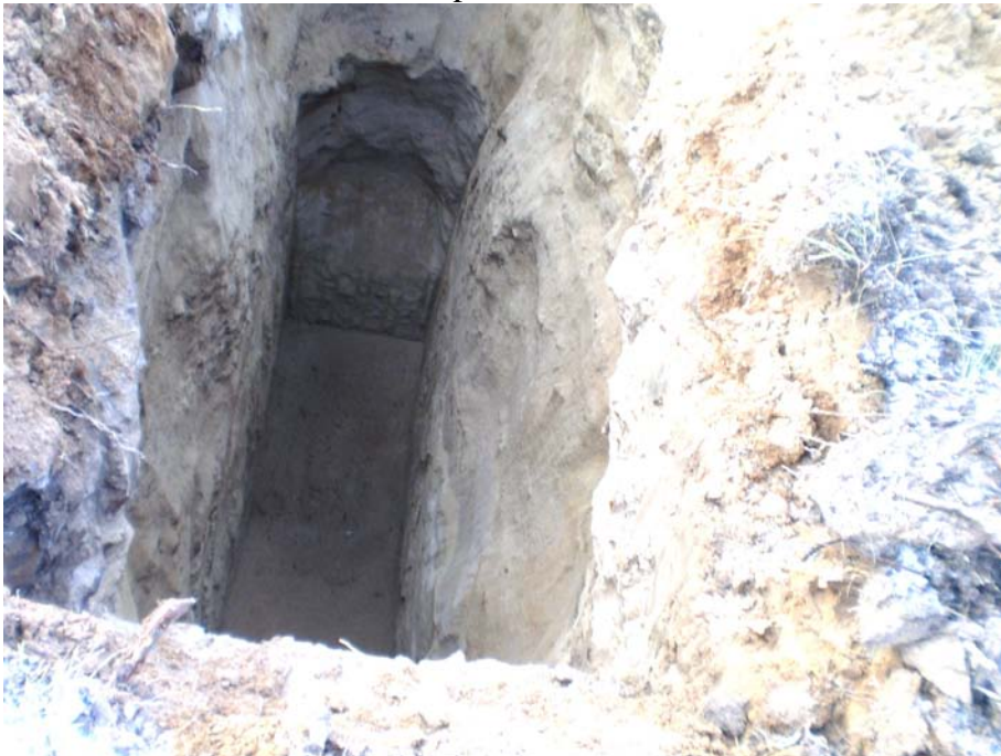
Photo 25 TH344 0.1-2' Gravelly clay 2-20' Gravelly sand
