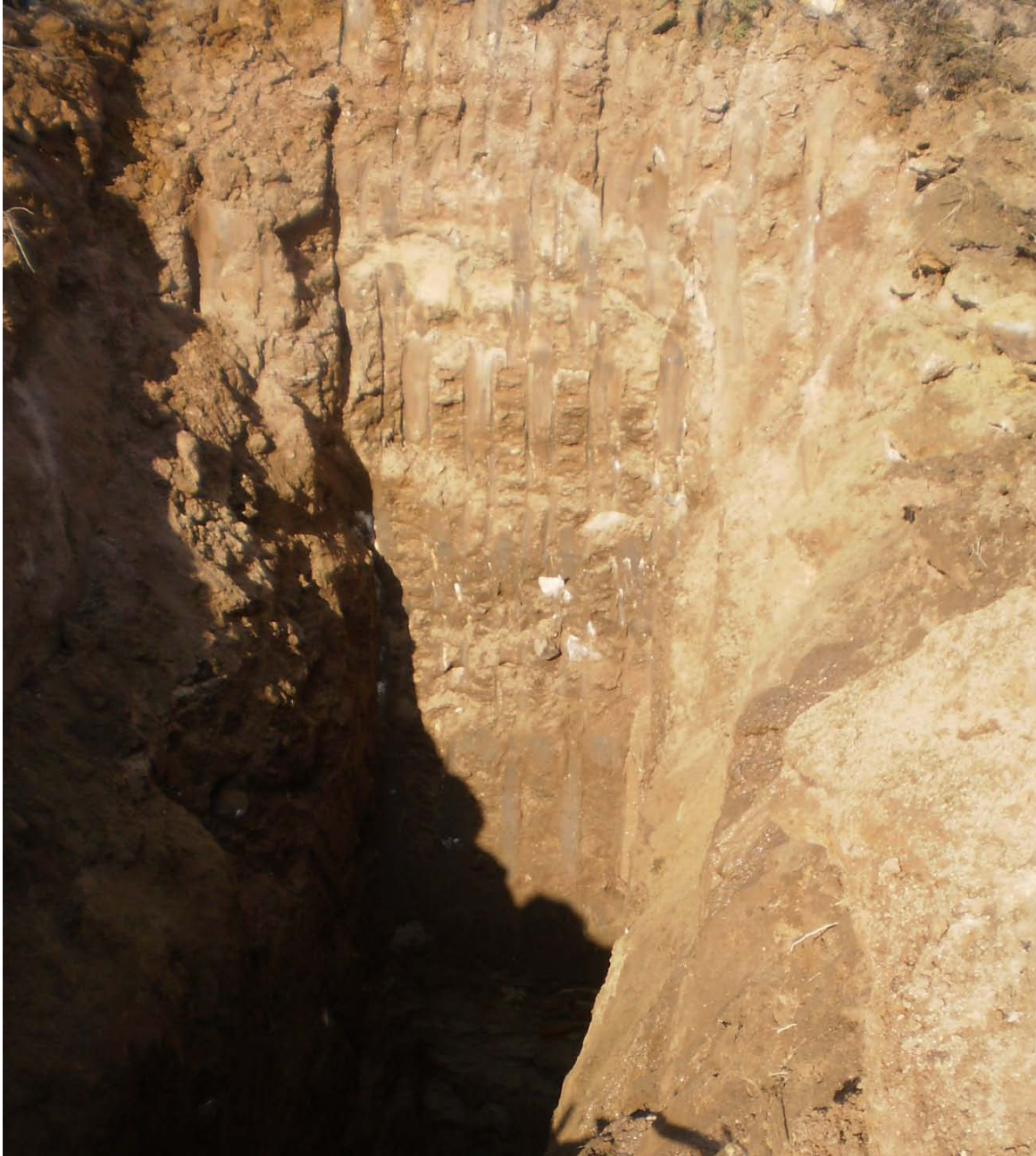
Photo 10 TH324 0.1-12' Gravelly clay 12-19' Sand 19-20' Gravelly coarse sand TH325 0.1-2.5' Clay 2.5-20' Sand
