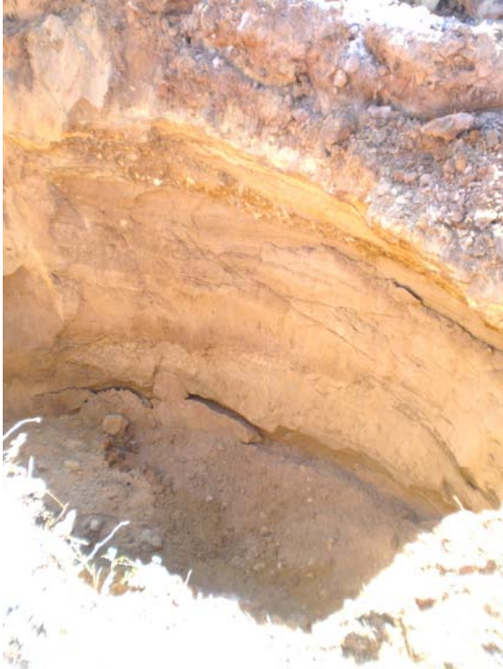
Photo 15 TH334 0.1-2.5' Gravelly clay 2.5-2.7' Gravel 2.7-20' Sand
