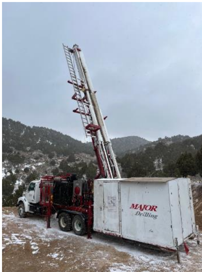
Figure 10.3 Surface Drill Rig at Big Hill
