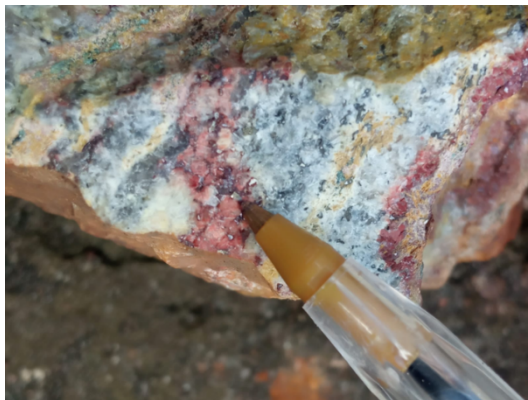
Figure 1: Sulphide mineralization hosted within hydrothermally altered granitic rock, showing disseminated sulphides associated with silicified and reddish potassic-altered zones.
