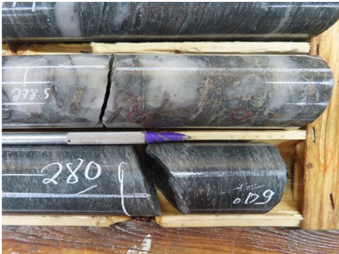
Figure 4: Mineralised tonalite contact with visible gold associated with quartz-pyrrhotite
