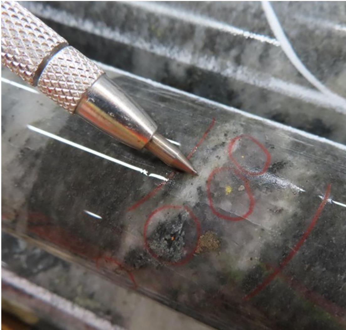
Figure 5: Mineralised vein is hosted in a moderately biotitized, silicified and albitized tonalite with tourmaline-quartz carbonate veins and local garnet porphyroblasts. (Hole EM21-207, 342.2m)
