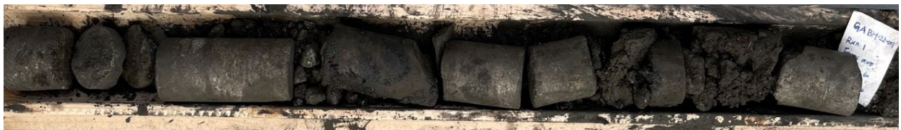
Figure 3. Massive sulphide cores from GABH-22-01 Backpack drilling hole at south section of Gamma Zone at Hawk Ridge Project
