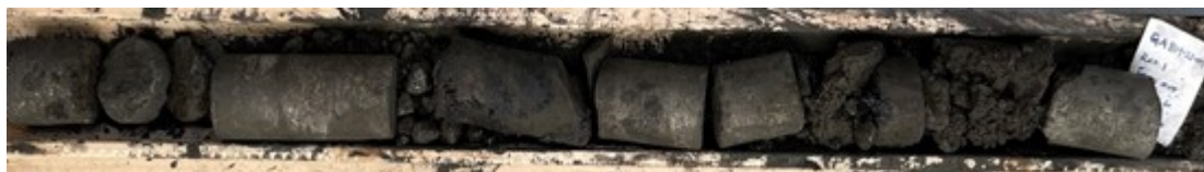
Figure 7 High-grade massive sulfide cores from GABH-22-01 Backpack drilling hole from Gamma
