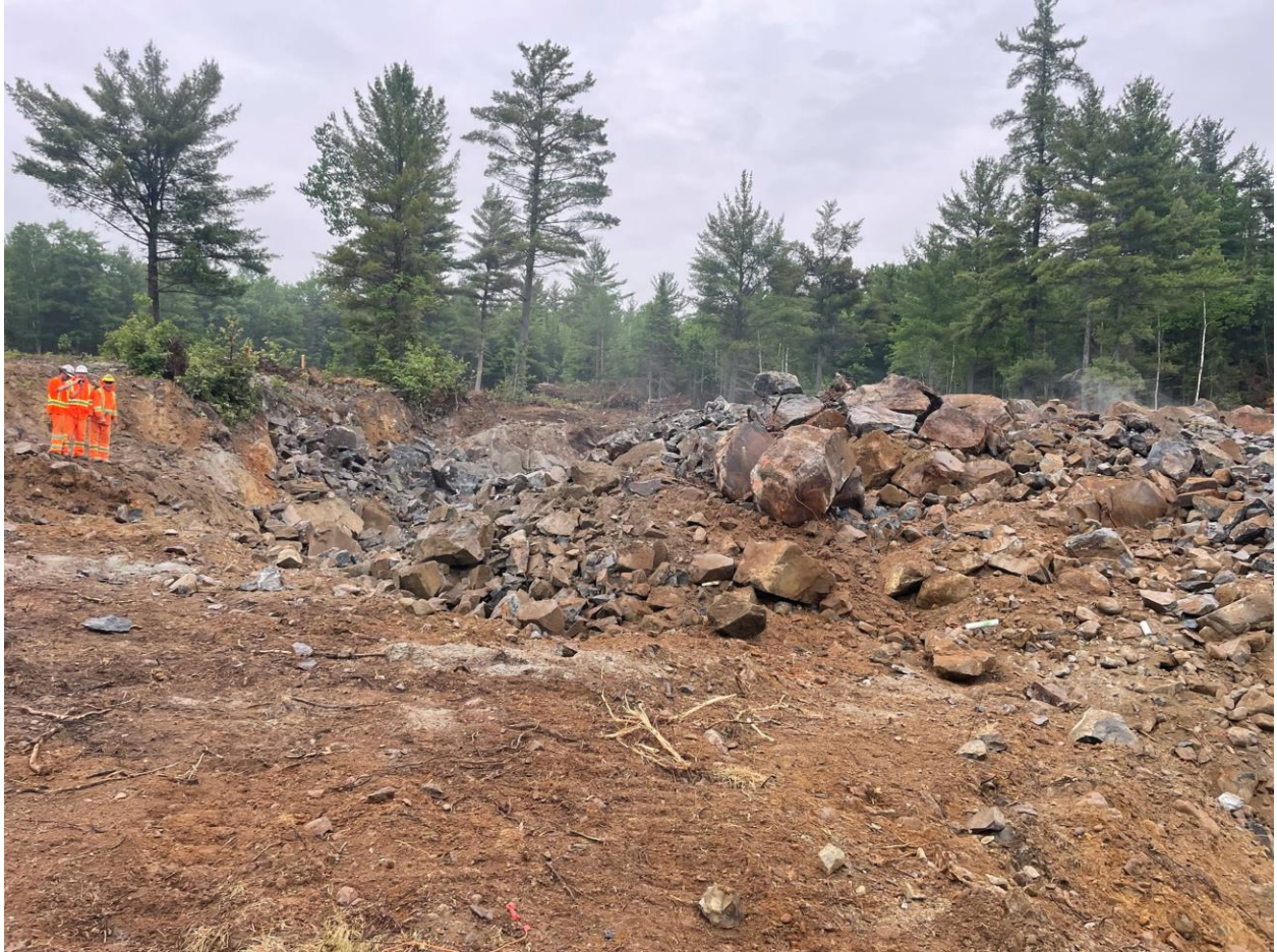
Figure 3. Photo of waste material from the 007 North pit after the blast that is removed prior to drilling and blasting of the targeted gold layer below.
