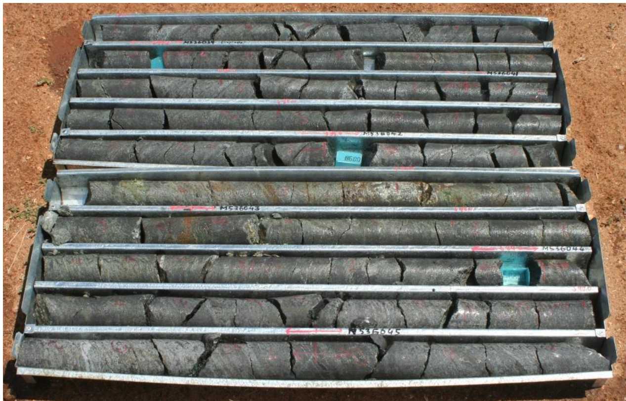
Figure 10-2: Core photographs of borehole MOLO-05 core (boxes 17 and 18) as supplied to CCIC by Energizer.
