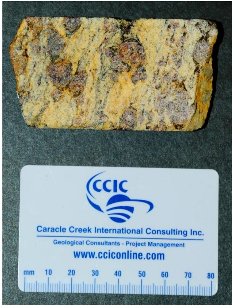
Figure 7-9: Garnet Gneiss in the footwall of Molo-4 at a depth of 132 m.
