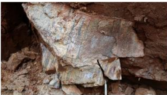
Quartzite-metachert from Trench TTR-18-17 – millimetre scale banding of magnetite within massive quartzite
