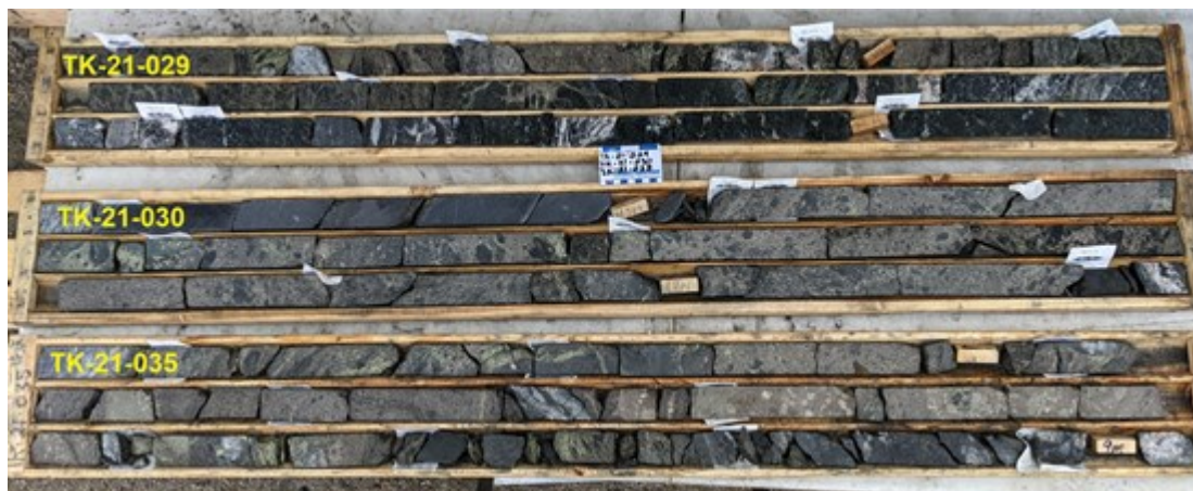
Figure 2. Massive and semi-massive magmatic sulphide intersections in holes TK-20-029, 30 and 35. Wall rock is tonalite, and hornblendite.
