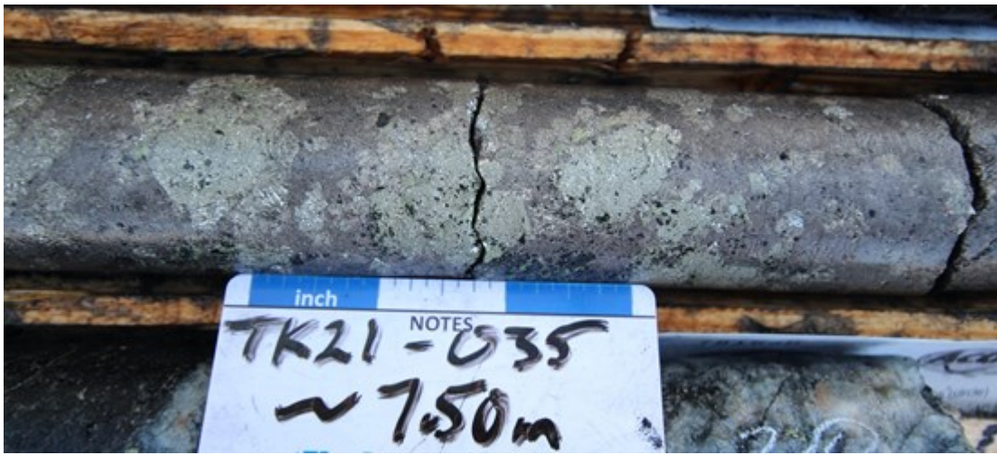
Figure 3. Closeup of coarse pentlandite eyes in hole TK-21-035.
