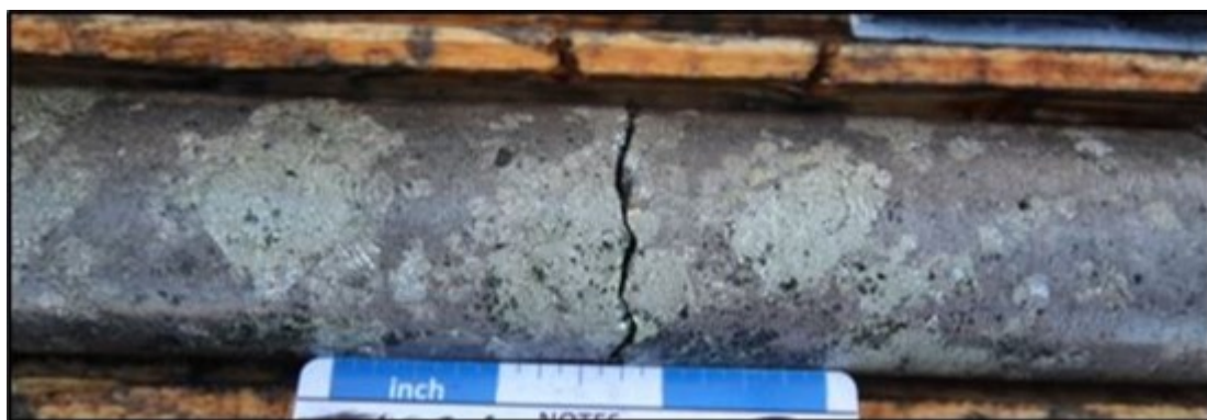
Figure 3. Coarse Pentlandite "eyes" in massive sulphide from hole TK21-035. This individual sample returned 11.9% Ni Eq (10.60% Ni, 1.47% Cu, 0.14% Co, 0.85 g/t Pd, 0.70 g/t Pt, 0.02 g/t Au).
