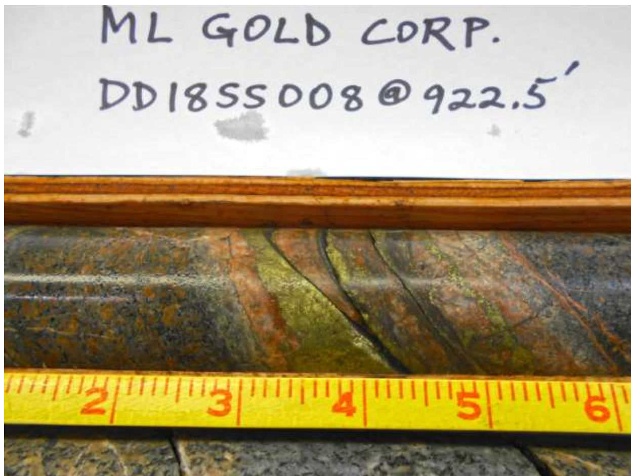
Figure 1: Chalcopyrite (copper) veining in structurally complex zone, current bottom of Hole 8 indicating mineralization is open to depth, drilling set to continue deeper.
