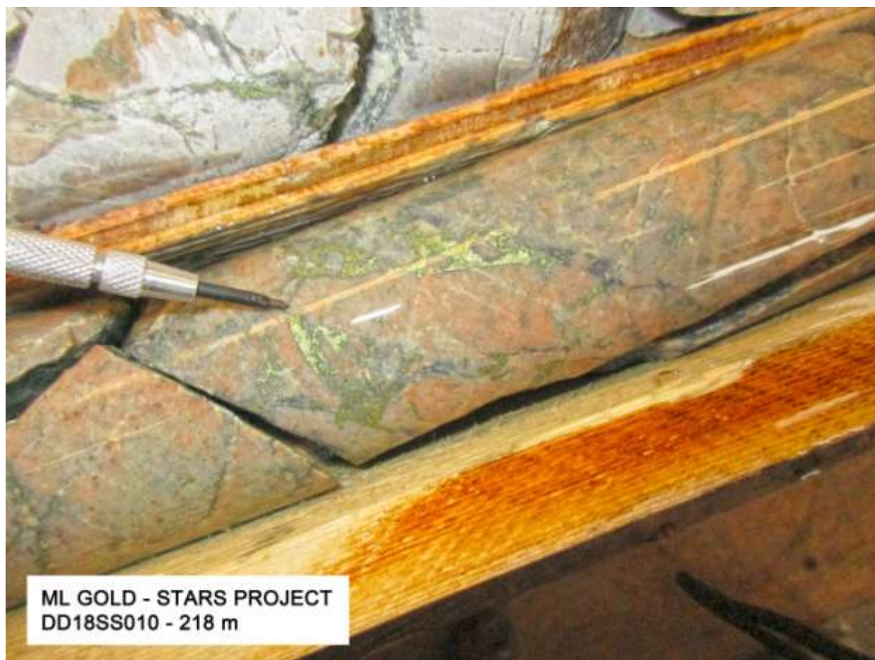
Figure 3: Potassically altered feldspar porphyry with coarse grained chalcopyrite disseminations – Sampled 12.2m @ 0.48%Cu
