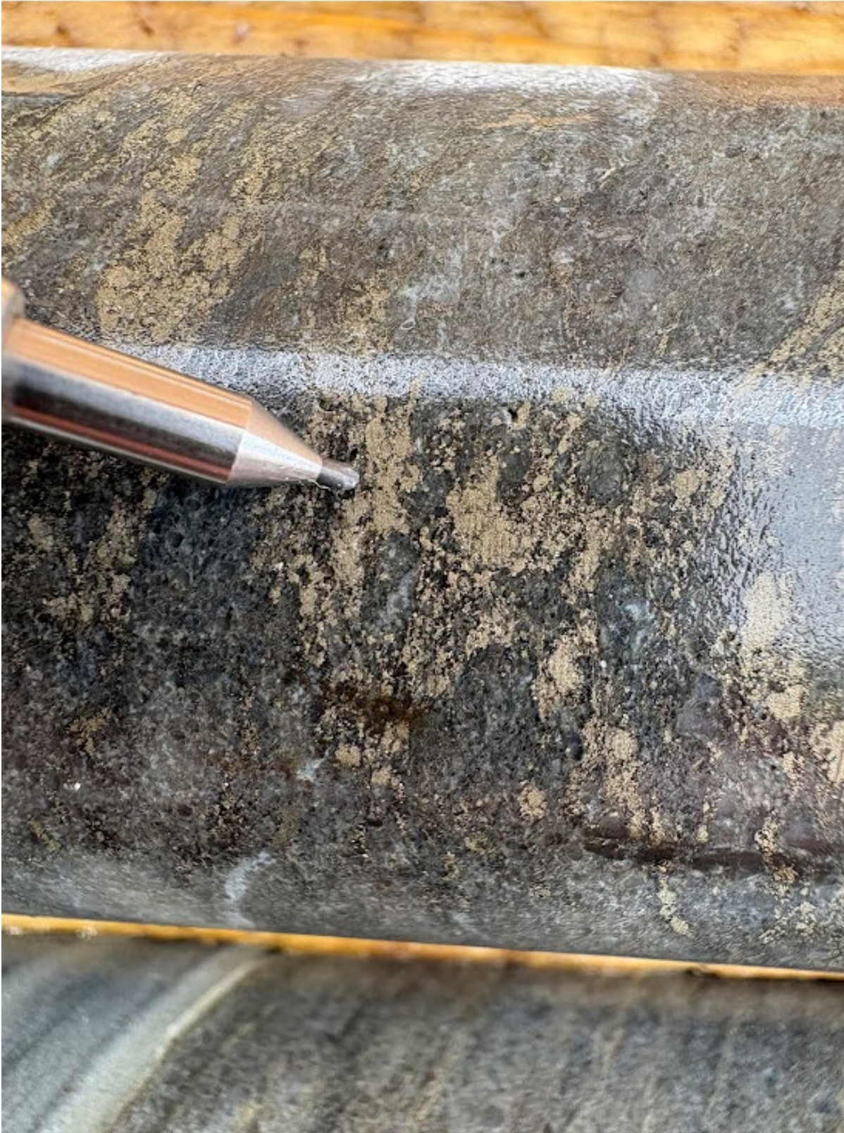
Figure 2: Stringers and Blebs of Strong Sulphide (Pyrite & Pyrrhotite with minor Chalcopyrite) Mineralization.
