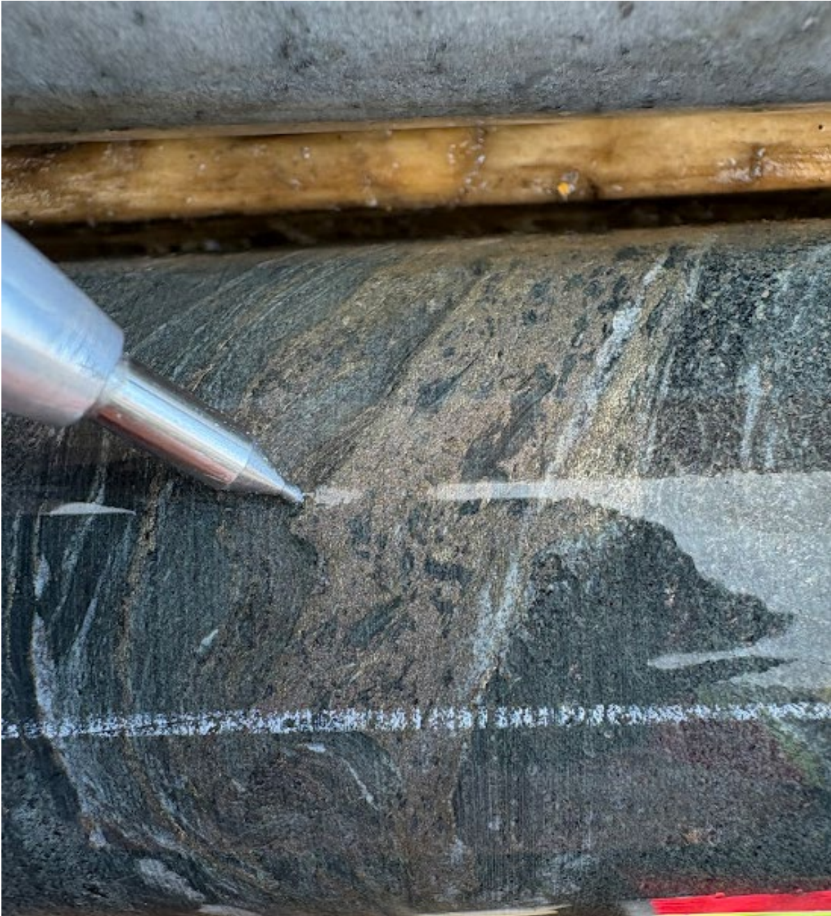
Figure 3: Narrow, Centimeter-scale Semi-massive Sulphide (pyrite and pyrrhotite) Band.
