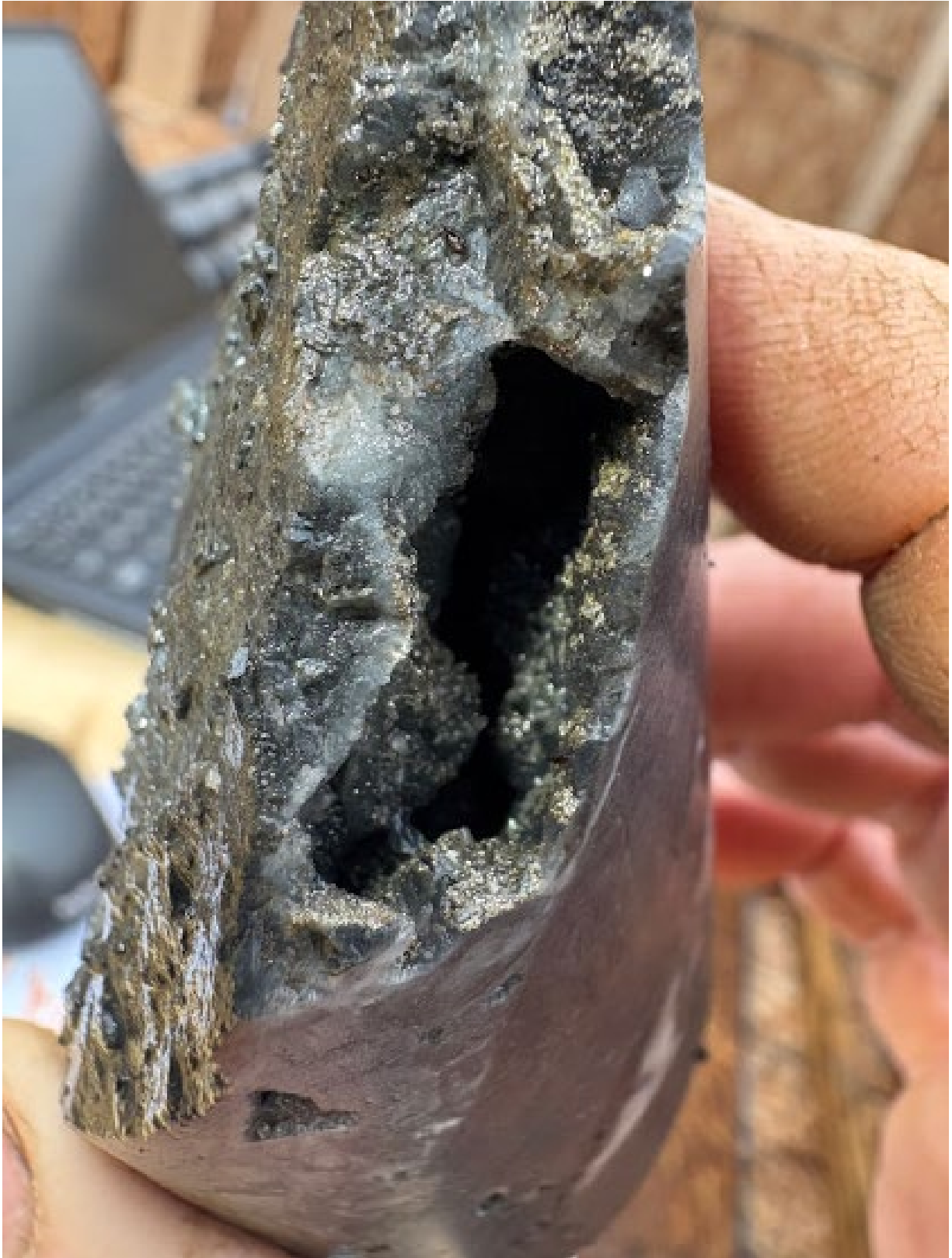
Figure 1: Disseminated Pyrite in a Vuggy Quartz Vein. Grey Coloured (smokey) Quartz Veins, Vugs, and Pyrite are Typical Indicators of a Gold Mineralization System.
