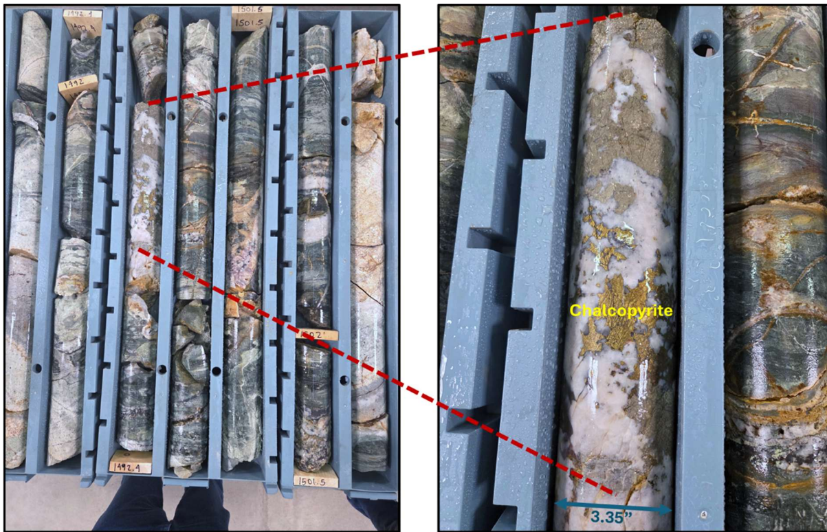
Figure-4. Example of copper sulfide mineralization intersected in NSM-16 from the recent HVA drilling program. For scale the drill core is 85.0 mm (3.345 inches) in diameter.
