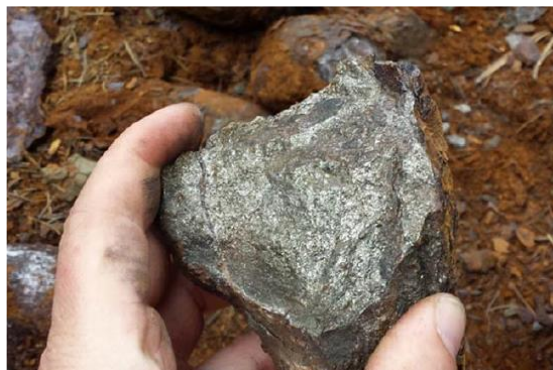
Massive sulphide from historic pit. 0.23% copper and 3.4 g/t silver
