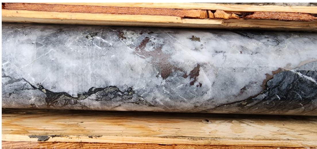
Close-up photo of sulphide mineralization intersected in holes AM23-07; galena, PbS (silvery grey) and sphalerite ZnS (brown). Width of view is about 10 cm.
