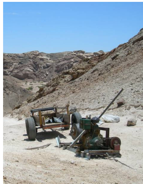
Pulley motor system to hoist drilling materials up the slope at Central Ida
