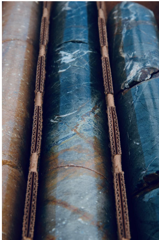
Figure 1 – Diabase showing prominent hydrothermal alteration (light green-gray + oxidation) against a rhyolite intrusion in drill hole MH-03.
