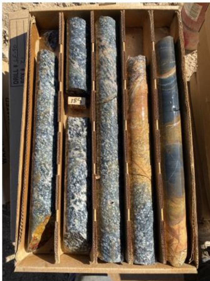
Figure 2 – Diorite and Diabase showing strong oxidation along intrusive contacts and local hydrothermal veins and fractures from MH-05.
