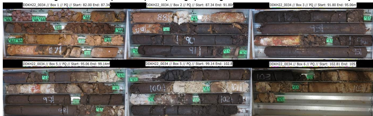
Figure 11 - An example of completed photograph collage of a diamond drillhole at the K.Hill Project.
