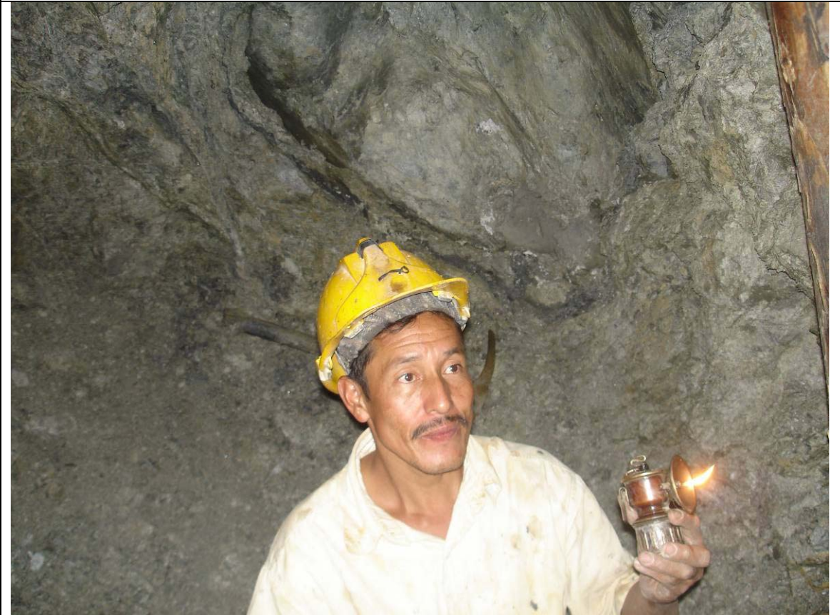
Plate 14.3. R. Dario of the Comunidad de Guayabales at a working face in the Encanto Zone within the Encanto Tunnel, Guayabales. Note the intensely altered and sheared nature of the Zone.
