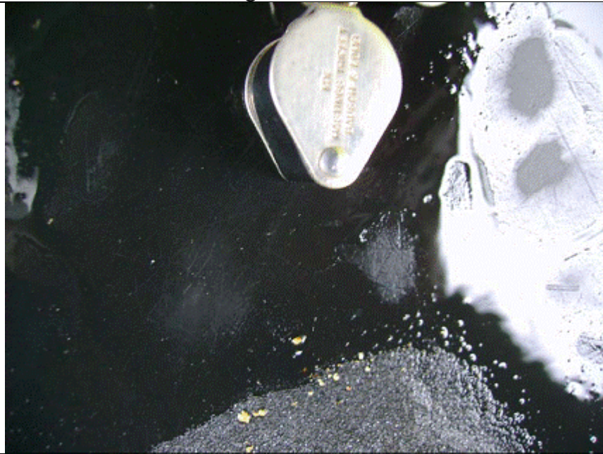
Plate 14.2. Panning is also used as a qualitative guide to grade at Guayabales. Coarse flakes of gold panned from crushed samples taken from El Encanto Tunnel indicate ore-grade material.
