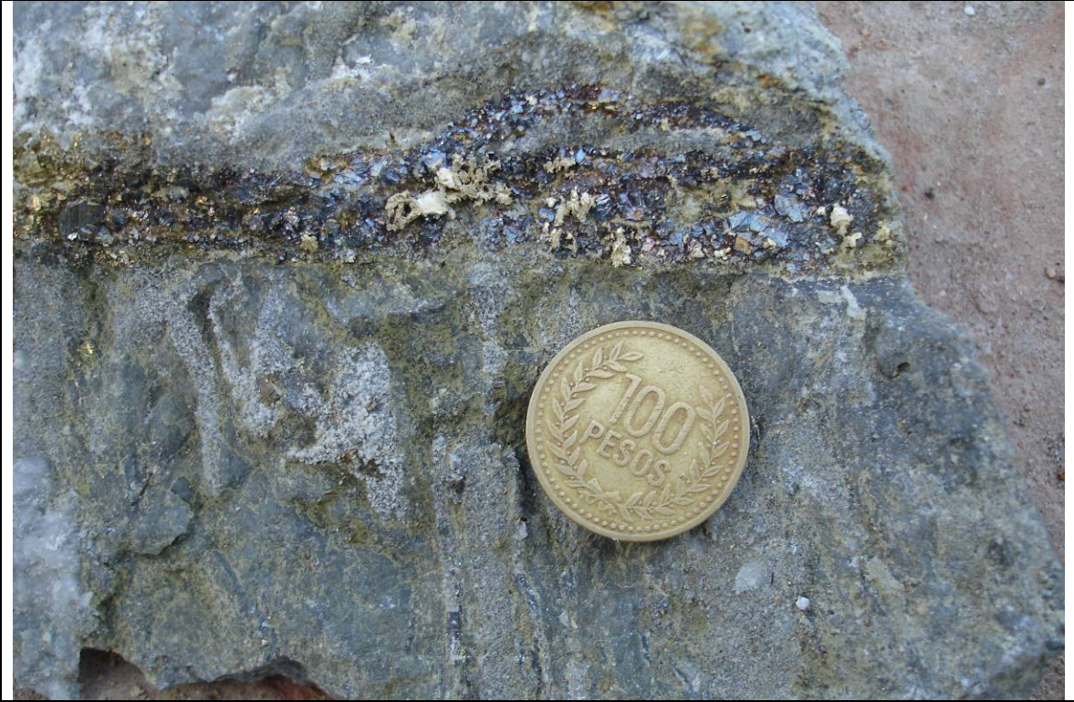
Plate 11.2. Early Pyrite veinlets oriented vertically in this picture are cut by a transverse veinlet containing pyrite, sphalerite, galena in this sample from the Azucena Mine at Guayabales. The base metal veinlet contains leaves of coarse gold/electrum just above and to the left of the coin. Both sets of veinlets show supergene chalcocite and covellite coatings over hypogene sulfides.
