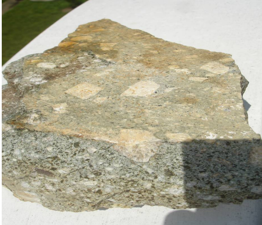
Plate 10.1. Marmato Stock “frog-eye porphyry” diorite porphyry with coarse plagioclase, hornblende and biotite with minor pyroxene phenocrysts in a microlitic matrix.
