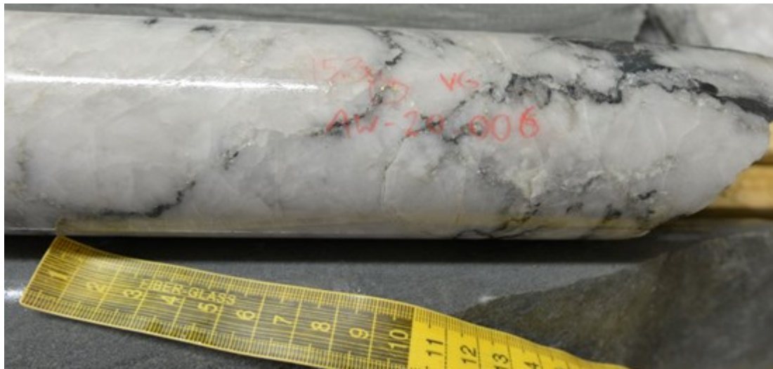
Figure 4: A representative sample of core showing visible gold in Hole AW-20-006 from 15.3m which intersected 0.9m @ 55.3 g/t gold
