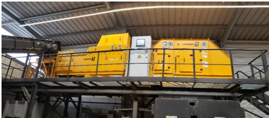
Figure 2. Steinert KSS sorter with XRT colour laser induction
