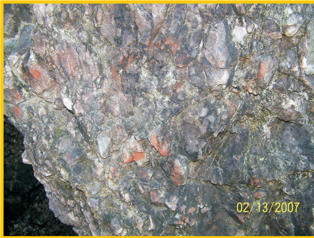
Figure 14a. Typical occurrence of the Au-Ag mineralized structure in the adit wall at the La Campana main showing. Notice the brecciation and the porphyritic andesitic fragments. The rock is heavily silicified, hematized and contains patches of epidote-chlorite. UTM coordinates: Easting: 428514; Northing: 2580870 (Zone 13N; WGS 84).
