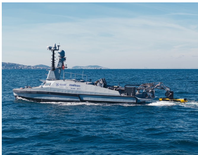
Figure 1: Kraken Robotics Demonstrates KATFISH Autonomous Launch and Recovery from a SEFINE RD-22 USV
