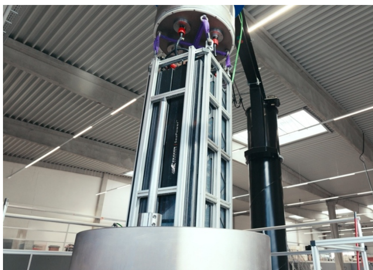
Figure 1: Kraken Robotics SeaPower batteries emerging from a pressure test system.
