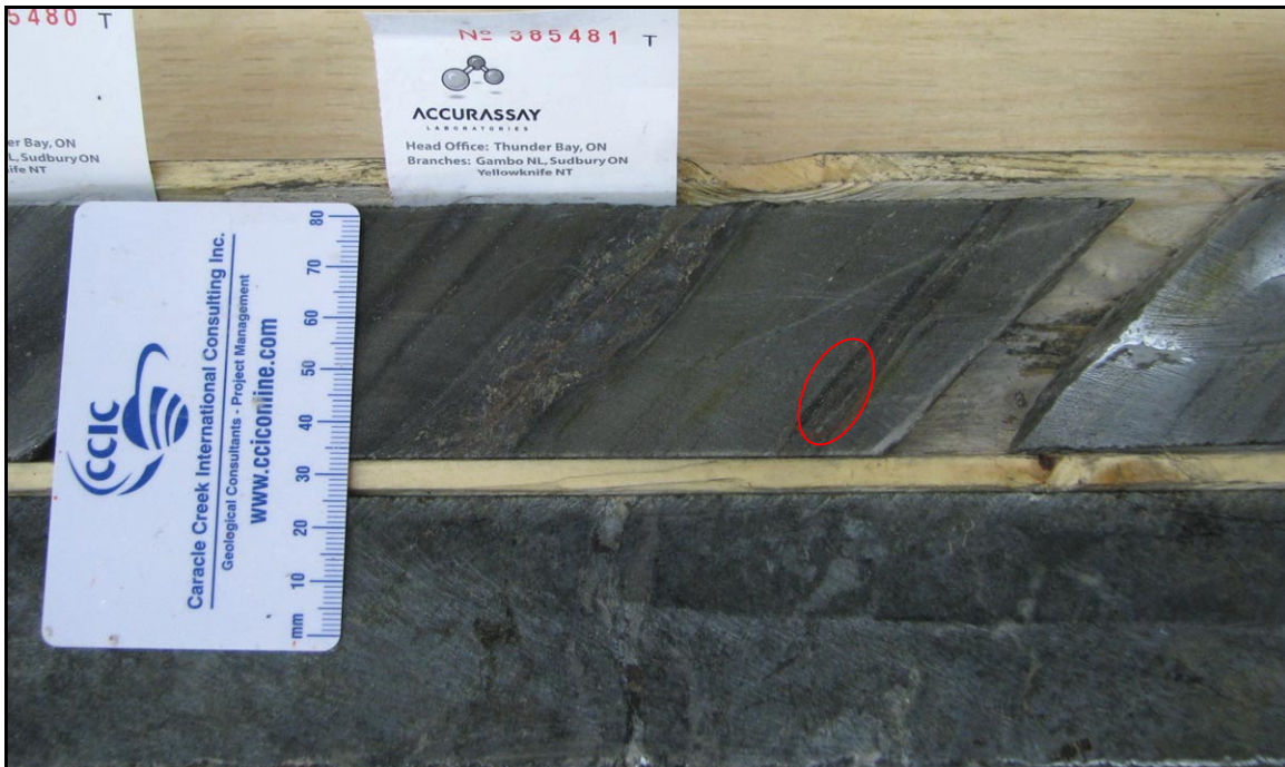
Figure 9-5. High-grade gold mineralisation with flakes of visible gold (VG) in a strongly altered section in felsic metavolcanic (biotite-muscovite schist) from the Main Zone (TL08-15, 50.8 m).
