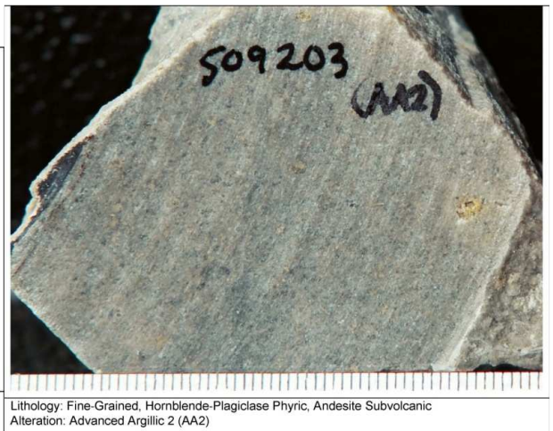
Photo 7. Advanced Argillic Alteration 2.
