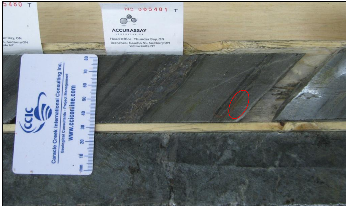
Figure 7-12. High-grade gold mineralisation with flakes of visible gold (VG) in a strongly altered section in felsic metavolcanic (biotite-muscovite schist) from the Main Zone (TL08-15, 50.8 m).
