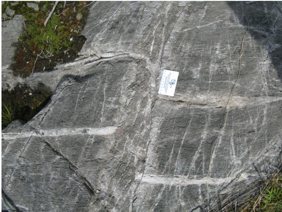
Figure 7-6. Chloritic biotite schist with 13cm wide fault zone, 352°/85, 16cm dextral displacement of feldspar vein. (8+85W, 4+30S, UTM 527879E, 5511200N, zone 15, NAD83).
