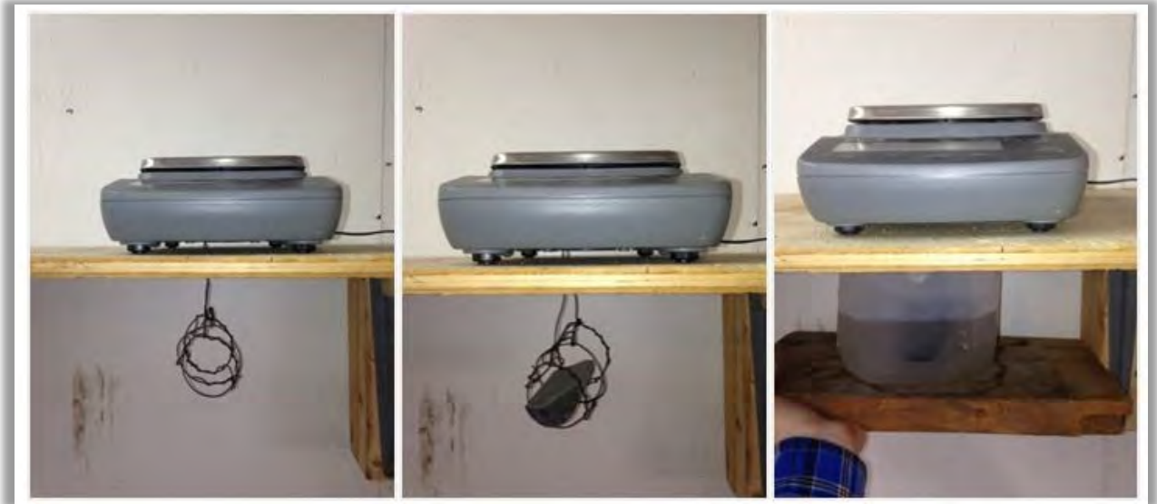
Figure 14.1 Specific Gravity Measurement Equipment Setup
