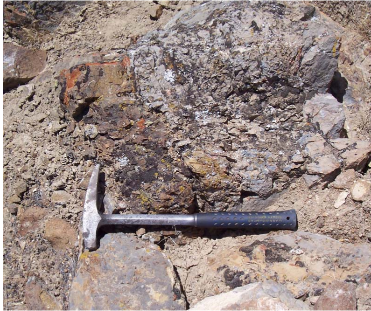
Figure 9.3.3.1: Photograph. Silicification as jasperoid vein (~ 20 cm wide) in brecciated Highway Limestone near intersection of north-south and northwest trending faults on the Iron Point Property. Exposure occurs along the basal contact of the Edna Mountain Formation. A recent rock chip sample returned a gold value of 1.175 g/t. Section 24 [T. 35 N., R. 41 E] JTK claim block area.
