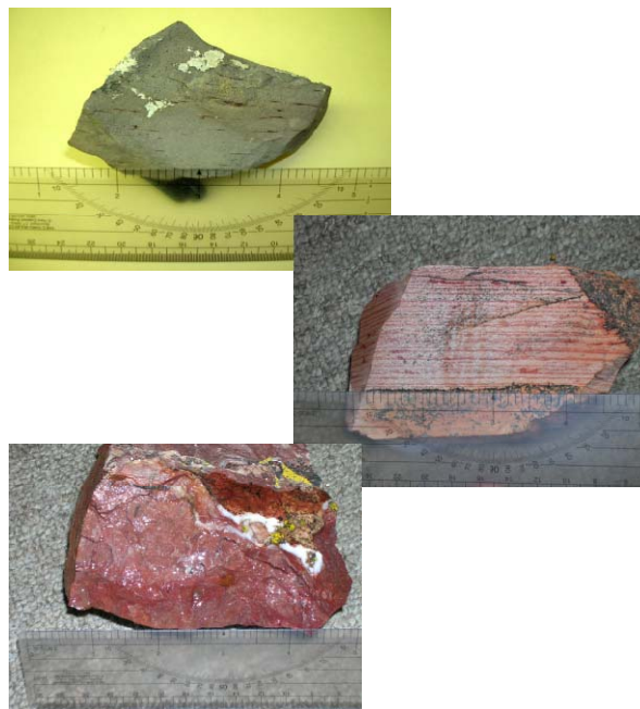
Figure 9.3.3.4: Photographs. Samples of Comus Formation alteration: 1) unaltered limestone 2) decalcified and 3) strongly oxidized silty limestone. Representative samples collected on the Iron Point Property.
