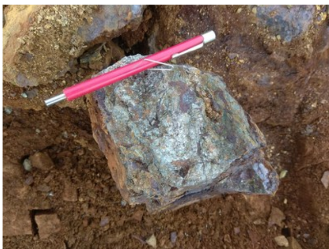
Photo 1: 104 g/t gold sample from breccia at Clive's Area at Ridge. Pyrrhotite, Chalcopyrite and Arsenopyrite. (CNW Group/Libero Copper & Gold Corporation.)
