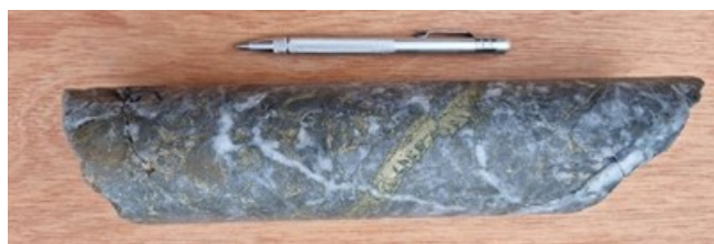
Figure 3 – 626m - Silicified dacite porphyry breccia: phyllic alteration with local potassic overprint. Several generations of quartz veining and chalcopyrite veining, with disseminated molybdenite and chalcopyrite. (CNW Group/Libero Copper & Gold Corporation.)
