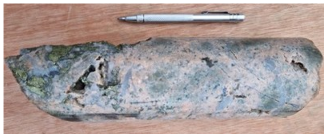
Figure 2 - 229m – Dacite porphyry breccia: intense potassic alteration (pink) mostly as halos around type A veinlets, quartz with chalcopyrite, molybdenite veinlets, disseminated molybdenite (grey speck) and chalcopyrite. (CNW Group/Libero Copper & Gold Corporation.)
