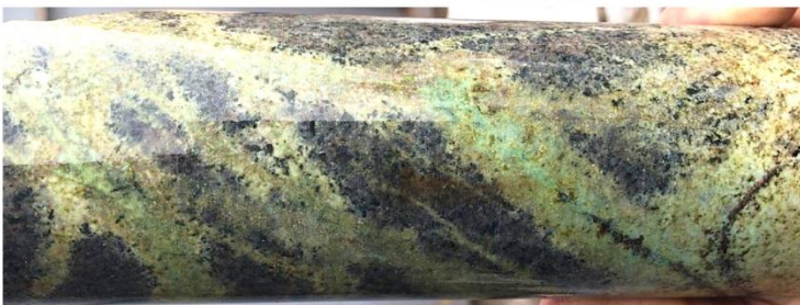
Figure 6: Illustrates copper oxide endoskarn mineralization within the Ccascabamba diorite sill.
