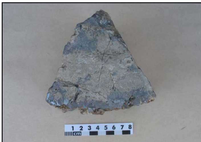
Figure 5: Specimen of sub-massive sphalerite and galena from Jubilee showing
