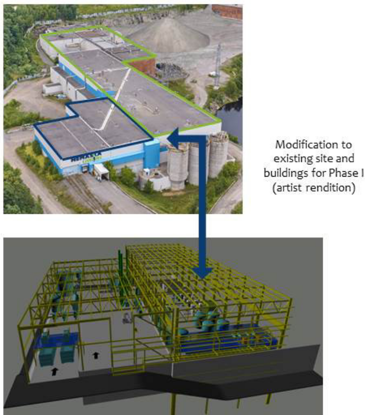
Figure 11 - Phase 1 Plant Layout
