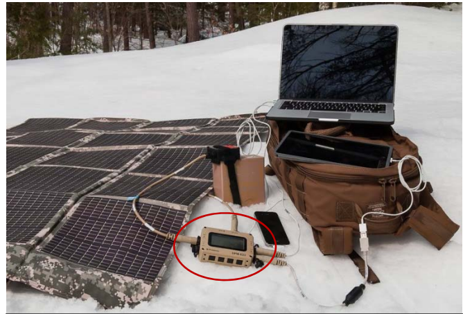
SPM-622 (circled in red) shown powering a laptop, tablet, iPhone & military battery, all from a solar blanket
