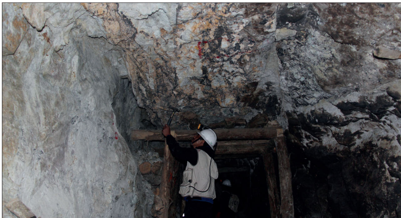
Figure 18: The San Jorge vein exposed on the Level 2 historical underground workings. In this exposure the vein is quartz dominant, crudely banded, with fracture limonite and manganese oxides. Primary sulphide minerals include galena, sphalerite and argentite.
