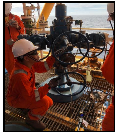
Figure 2: Technicians take pressures during inspection.
