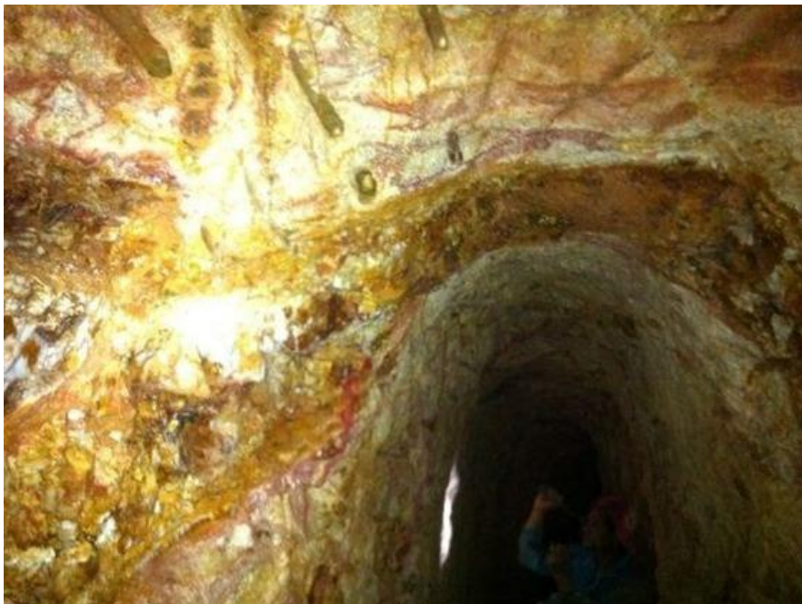
Figure 1 Inside the CZ Gold tunnel showing vein and stockwork and adit.
