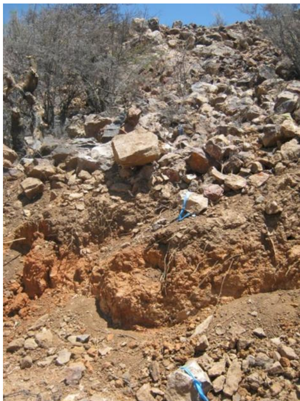
Figure 24. Blue Flagging Marks Alignment for Drill.
