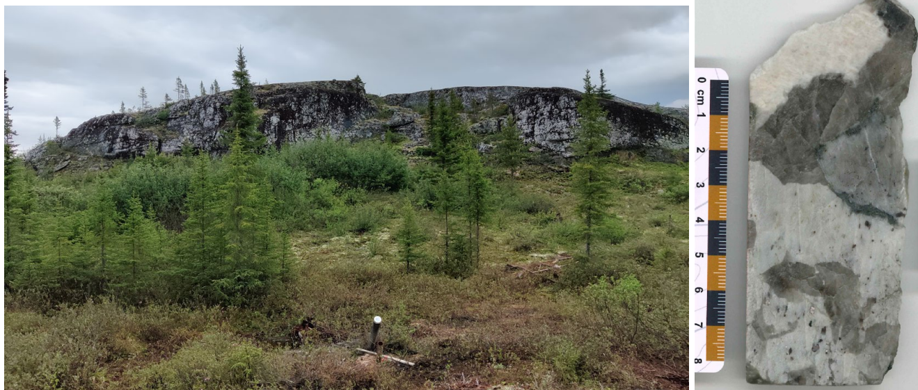
Figure 30: Principal spodumene pegmatite body outcropping at CV5 with drill hole CF21-001 in forefront (left); typical mineralization from drill core at CV5 (right).
