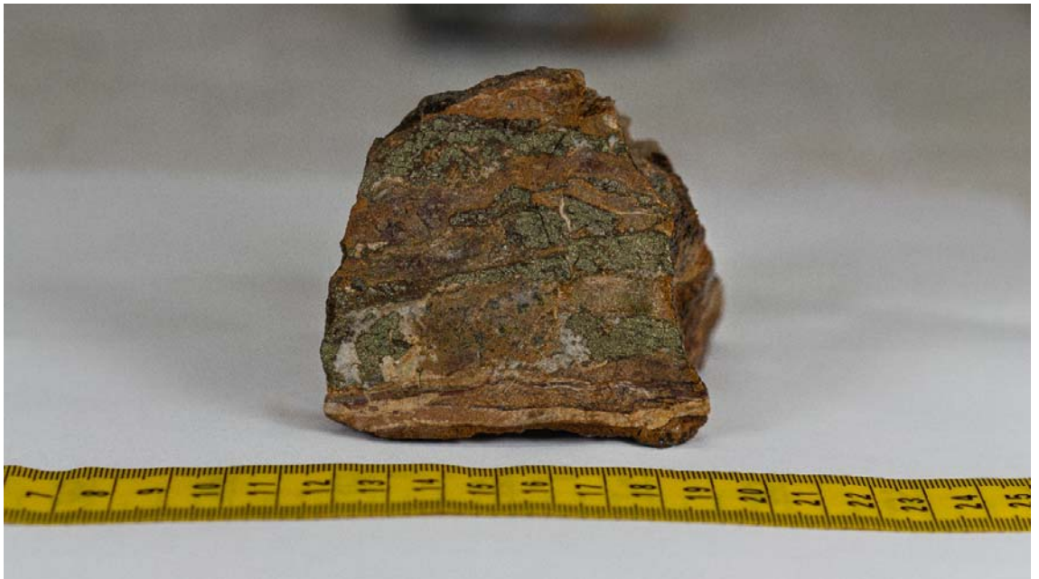
Chalcopyrite mineralization hosted in a potassic, hematite, and carbonate altered porphyritic syenite found at outcrop on “Rock Island I”; a new showing ~800 metres NE of Burgundy Ridge and ~500 metres NW of the Telena Zone.
