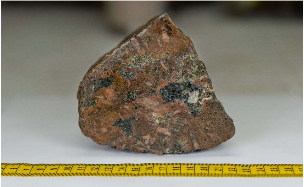
K-feldspar altered megacrystic syenite with chalcopyrite mineralization found in outcrop at “Rock Island II”, a new showing ~470 metres NE of Burgundy Ridge exposed by rapidly receding glaciers.
