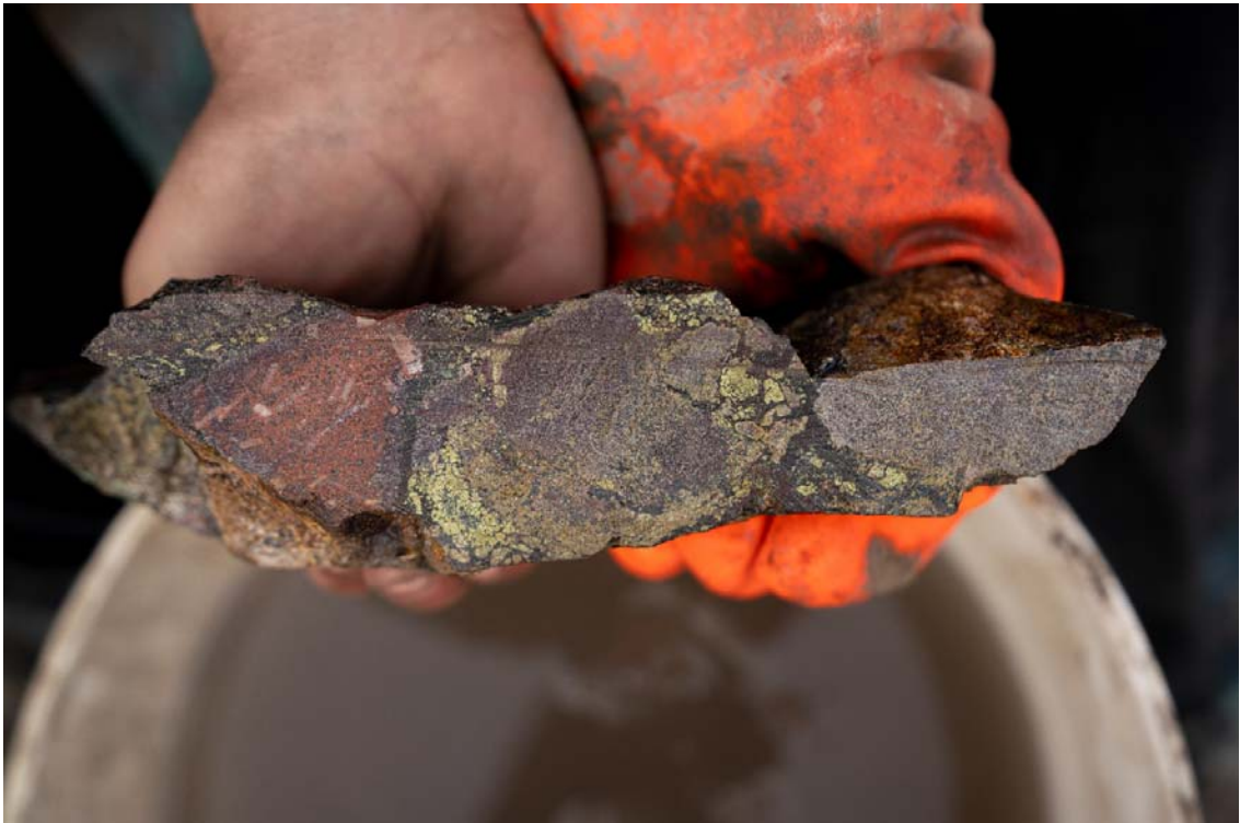
Representative sample from Ridge Zone Channel Sample #1 (“BRCH19-001”); a 37-metre continuous channel sample taken on surface at the “Green Rock” showing. Chalcopyrite, sphalerite, and pyrite cement of hydrothermal breccia is observed. This new showing is ~350m south of drill pad “A-1” along the Burgundy Ridge Trend. Assay results are pending.
