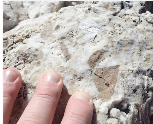
Left: Silicified green volcanic (Dacite). Malachite and chalcopryite (approx. 1-2% disseminated) are hosted in volcanics. Late quartz veining crosscuts and a quartz veining cross-cuts volcanics is locally hematite manganese stained.
