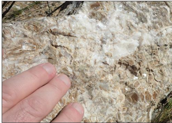
Below: Hydrothermal breccia. Silicified red volcanic clasts supported in fine-grained white quartz
