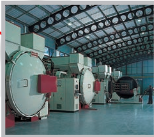
Solution and ageing heat treatment is used to strengthen the implant.
